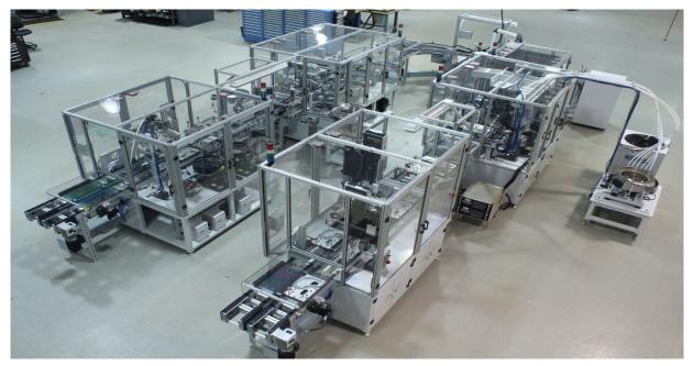
**Battery Plate Manufacturing System-** Inline process for carbon foam/lead plates. Machine cut foam to size, added lead grid plates and attached them through IR heating. Single plates were inspected and then unloaded on a conveyor. This machine produces 20-plates every 30-seconds.
